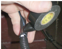
TAPE THE SPLIT LOOM (NOT SUPPLIED)
